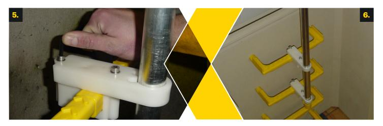
Tighten 4 screws with 5mm Allen key.
